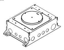
RFBA 10-Gang Round Floor Box, 6.25" Depth - Steel floor box designed for above grade installations. Features 10-gangs of box capacity with at least 2 1/2" available behind device plates. Fully adjustable before and after concrete pour. Designed for carpet, wood flooring, tile, terrazzo and polished concrete applications. Use with Evolution™ Series 8" round covers.
