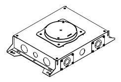
RFBA 4-Gang Round Floor Box, Standard 3.75" Depth - Steel floor box designed for above grade installations. Features 4-gangs of box capacity with at least 2 9/16" will able behind device plates. Fully adjustable before and after concrete pour. Designed for carpet, wood flooring, tile, terrazzo and polished concrete applications. Use with Evolution™ Series 6" round covers.
