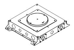
RFBA 6-Gang Round Floor Box, Standard 3.75" Depth - Steel floor box designed for above grade installations. Features 6-gangs of box capacity with at least 2 9/16" will able behind device plates. Fully adjustable before and after concrete pour. Designed for carpet, wood flooring, tile, terrazzo and polished concrete applications. Use with Evolution™ Series 8" round covers.
