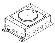
RFBA 10-Gang Round On-Grade Floor Box, 6.25" Depth - Steel floor box designed for on-grade installations with a fusion-bonded epoxy for use on metal reinforcement bar and related accessories before encapsulating in concrete. Features 10-gangs of box capacity with at least 2 1/2" available behind device plates. Fully adjustable before and after concrete pour. Designed for carpet, wood flooring, tile, terrazzoand polished concrete applications. Use with Evolution™ Series 8" round covers.
