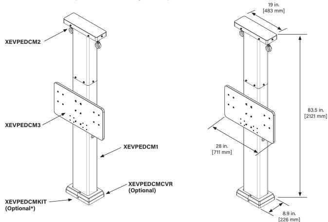
\*XEVPEDCM1 includes mounting expansion bolts. XEVPEDCMKIT can be purchased for fresh concrete pour applications
