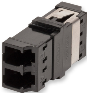
Fiber Optic Adapter, LC Duplex, Non Keyed/Non Keyed, Reduced-Flange Mount, Ceramic Sleeve, (OM4+/OM4/OM3/OM2/OM1/OS2), black
