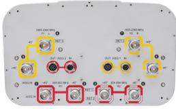
8-port sector antenna, 2x 698–803, 2x 824–894 and 4x 1695–2360 MHz, 65° HPBW, 3x RET and low bands have diplexers. Internal SBT's on first LB(Port 1) and first HB(Port 5).
