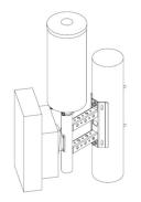
Small Cell 4G-5G Side Pole Mount - One Sector (1 antenna / 1 radio)
