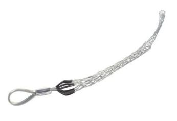
Multi-Weave, Rotating Eye. Cable Diameter - 3.000-3.490-inch, Mesh Length - 54-inch, Eye Diameter - 1 7/8-inch, Break Strength - 48,000 lbs, Aluminum.
