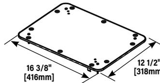
**Bare Concrete/Terrazzo Trim Ring** – Nonmetallic ring for use with bare concrete and terrazzo floor applications.
