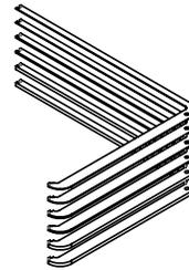
**Tile Shim** – Used for floor coverings greater than 3/16" [4.7mm]. The EFB610-TS allows the finished cover assembly to be flush with the finished floor. Includes one (1) 1/16" [1.6mm], one (1) 1/8" [3.2mm] and one 1/4" [6.4mm] tile shims for 7/16" [11.1mm] of upward adjustment.
