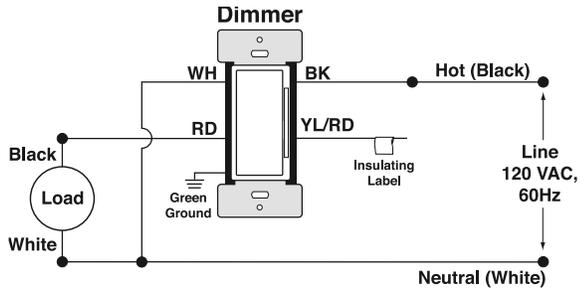
**THREE-WAY WIRING DIAGRAM**
