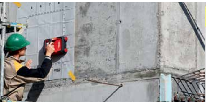
Non-destructive inspecting of concrete structures, e.g. locating reinforcement or post-tension cables. (Post-tension cable inspection applies to PS 1000 only)
