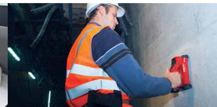
Measuring of concrete coverage for acceptance inspections, renovation work and quality checks.
