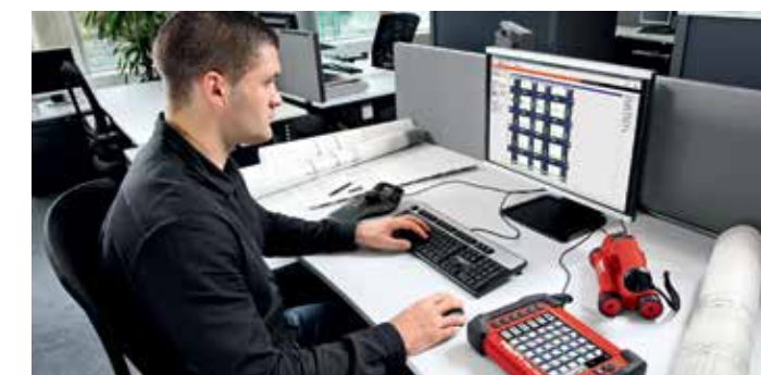
Rebar detecting and verifying for acceptance inspections, changes of building use or post-installed rebar connections.
