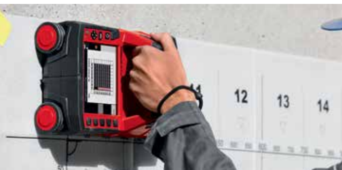
Locating objects in concrete structures before drilling penetrations or breaking out openings.
